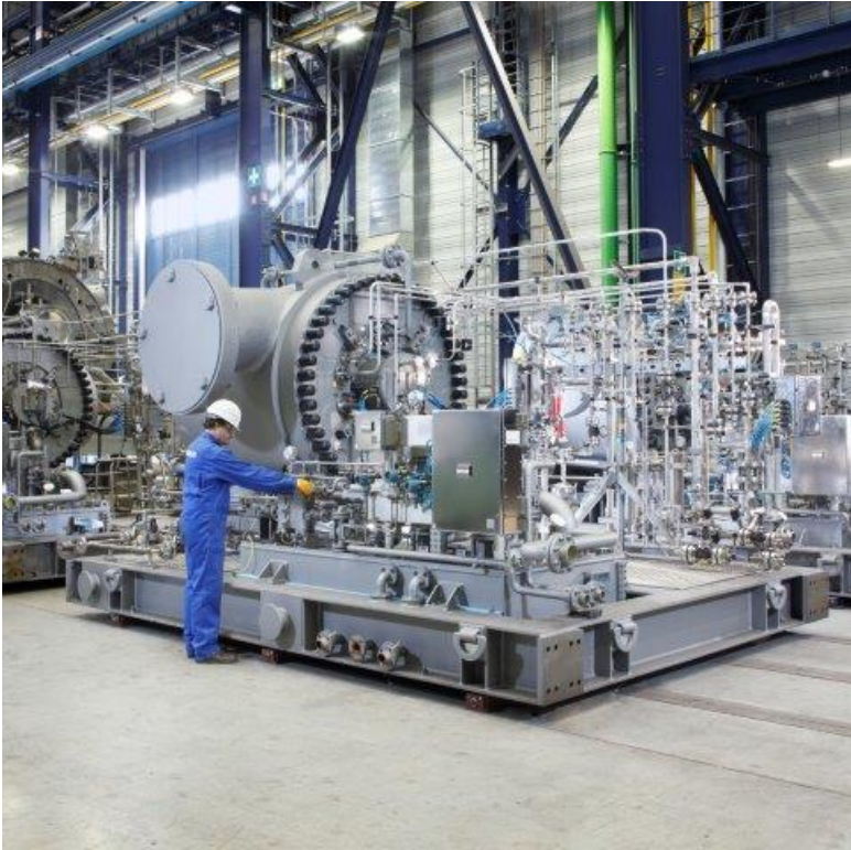
Siemens STC-SV single-shaft pipeline compressor.
