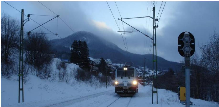
Both pictures: Vectron 193 923 at the beginning of 2012 during winter testing on the Iron Ore Line. Preliminary homologation was issued for the Swedish network after the locomotive successfully completed testing under winter conditions in northern Sweden.
