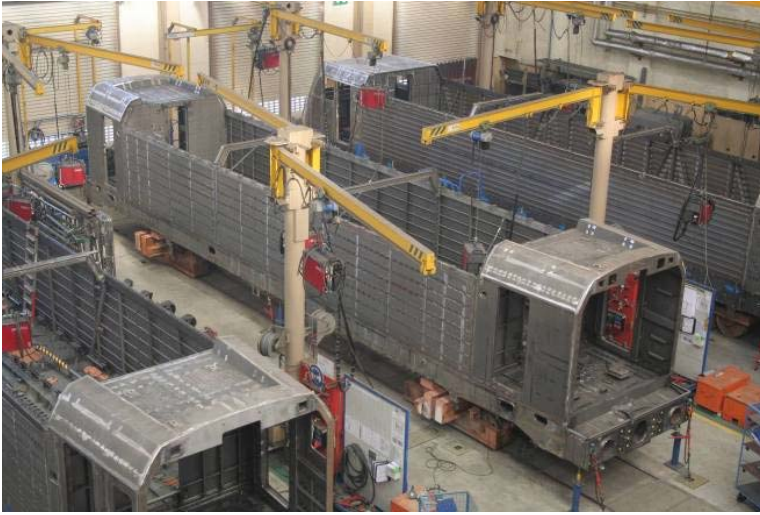
Fig. 5: Vectron car body
