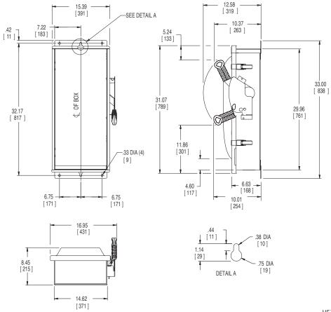
No knockouts in enclosures. Dimensions shown in inches and millimeters ( ). Dimension shown accurate to  $\pm$   $^{1/8}$  inch.
