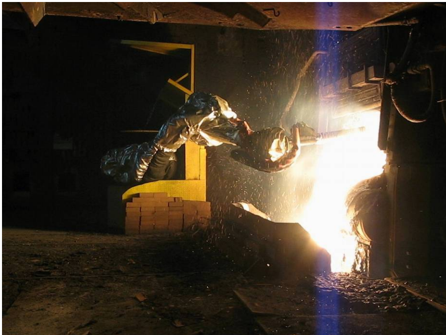
The Siemens LiquiRob robot system in action at the electric arc furnace of SAM Neuves-Maisons, Riva France
